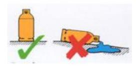
Cylinders should be placed upright and outside the confines of the cooking tent so the cylinder valve is more accessible in the event of a fire. Allow enough hose for this. Bottles should not be kept under a cooking table as, should a fire start, you cannot get to the bottle to turn off the supply without going under the fire itself.
